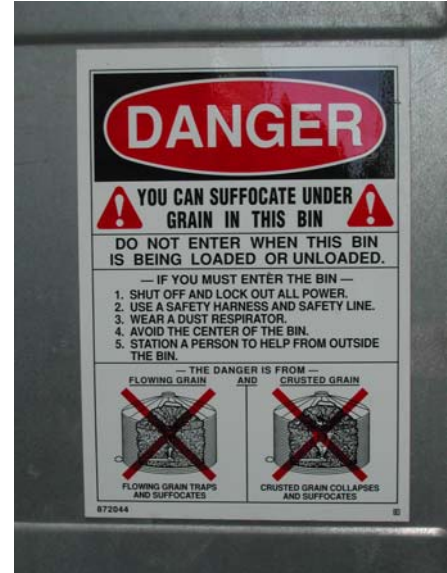
Figure 3. Confined Space warning sign on bin door
